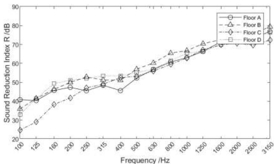
Figure 5. Sound Reduction Index R (dB) of the construction solutions listed in Tab. 2.
