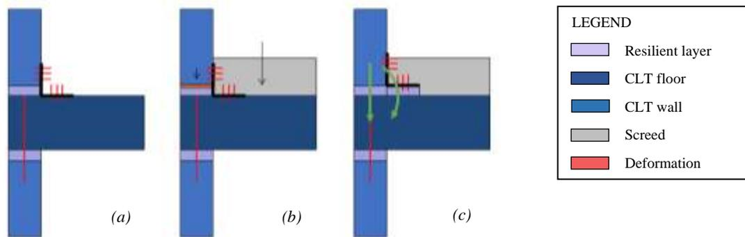
*Figure 2: Schemes of CLT junction with the soundproofing profiles: (a) resilient stripes are places between timber elements; (b) the structure is loaded by permanent non-structural loads and the resilient layer is compressed; (c) the resilient layer is placed also below the metallic connectors, modifying the load transmission.*
