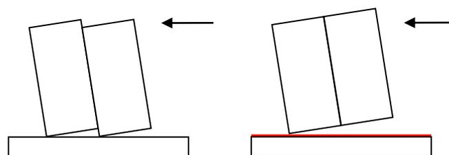
*Figure 3: Scheme of the test results achieved at the Karlsruhe Institute of Technology. Left: the junction was assembled with no resilient interlayer and the connection correctly dissipates energy. Right: the resilient interlayer prevents the junction from dissipating energy.*
