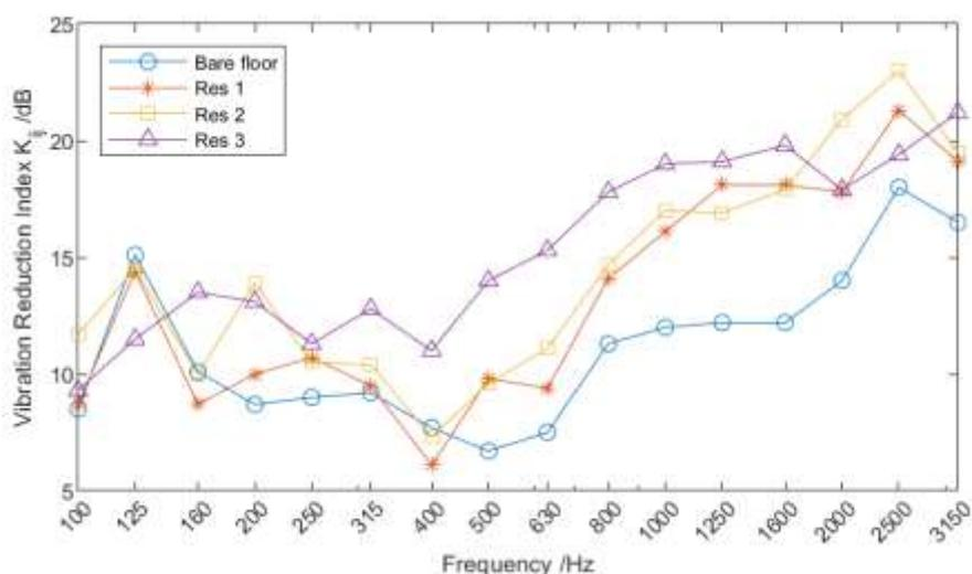
Figure 1: Vibration reduction index  $K_{ij}$  (dB) measured on a wall-floor junction without (bare floor) and with (Res1/2/3) the interposition of a resilient material, after (Morandi *et al.*, 2018).
